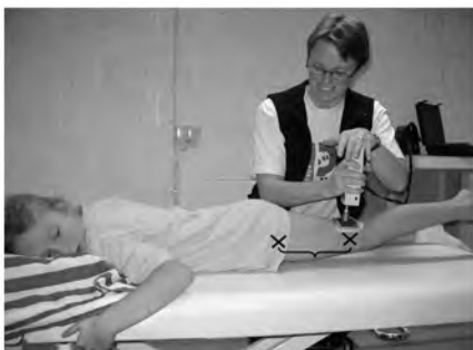
Figure 2.3. Measurement of hip extension with the Chatillon dynamometer. Lever arm indicated with X.
